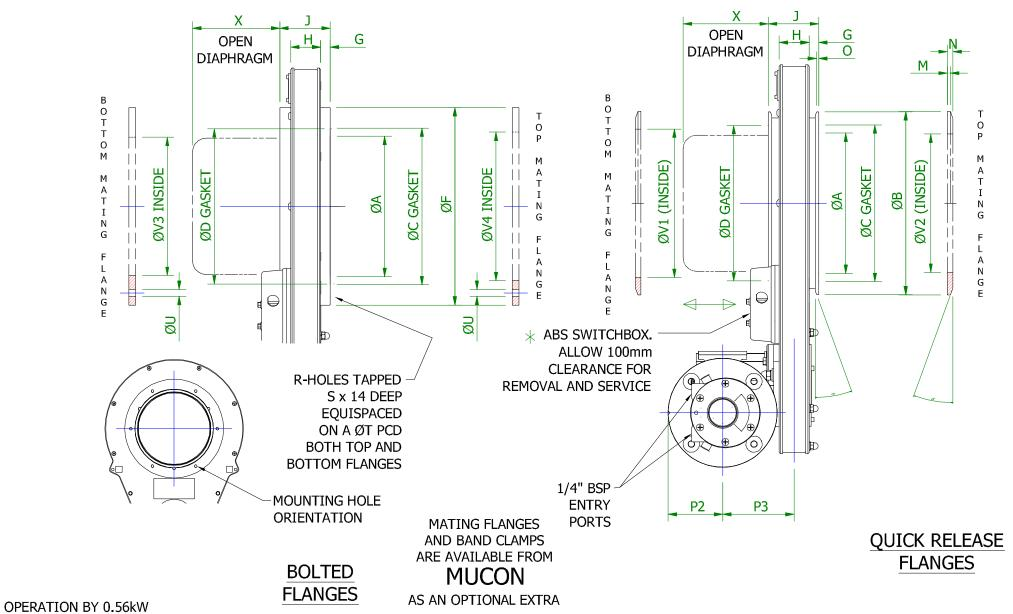
3000rpm, REVERSIBLE AIR MOTOR USING 1000 l/min OF LUBRICATED COMPRESSED AIR @ 5.6 bar. PORT SIZES TO BE 1/2" BSP (min) FOR REQUIRED AIR FLOW.
