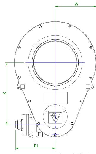
VALVE FITTED WITH OPEN, CLOSED & TRICKLE POSITION INDICATOR SENSORS.
